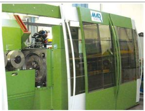
Coil-to-bar peeling machines to produce high quality peeled bars from 5 to 60 mm dia, cylindrical and tapered.
