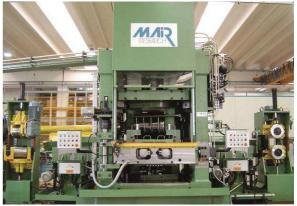
Bar centerless grinding machines to process bars from 2 mm up to 130 mm dia.
