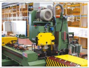
Multiple saw to cut tubes and bars max OD 240 mm. The cutting units are adjustable and provide the simultaneous and automatic cutting operation of tubes and bars of different length.
