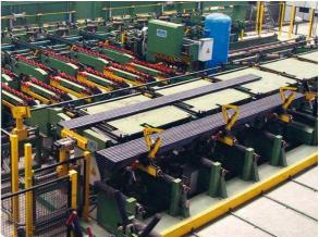
Single saw to cut tubes and bars max OD 230 mm. The sawblades, together with an accurate control of the cutting and feeding speeds controlled by the automation system, assure the best cutting quality, free from any burr and defects, for all steel grades and non-ferrous materials.
