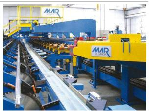
Ten-roll tube straighteners handling tubing with dia. 10 upto 250 mm, with straightening speed up to 300 m/min.
